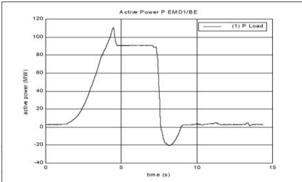
**Fig. 3:** Active power of the pulsing load at 450 GeV.
