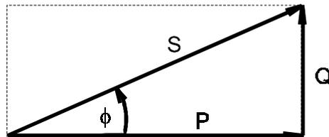
Fig. 1: Phasor diagram of active, reactive and apparent power.
