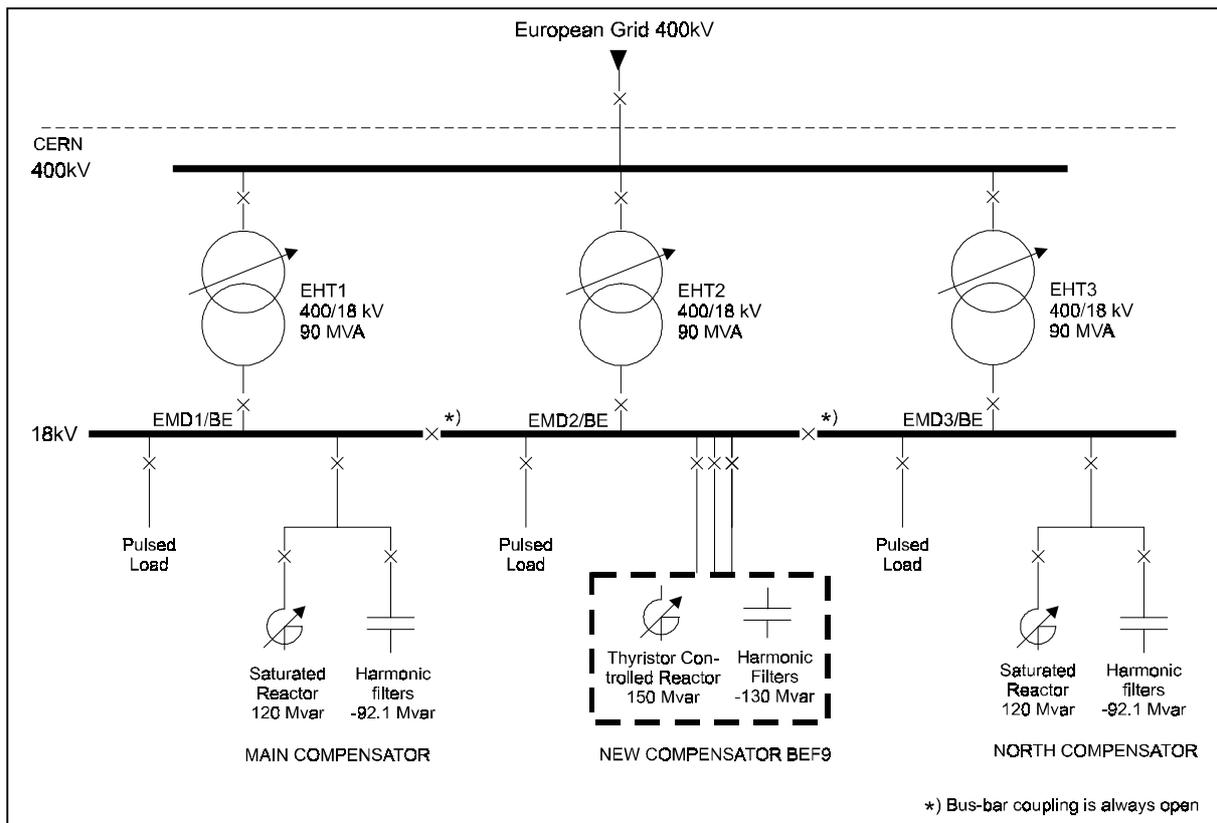
Fig. 2: Simplified layout of the SPS pulsed network.
