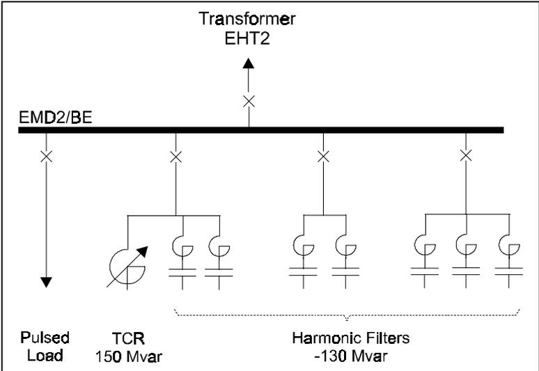
**Fig. 6:** General layout of the new Static Var Compensator BEF9.
