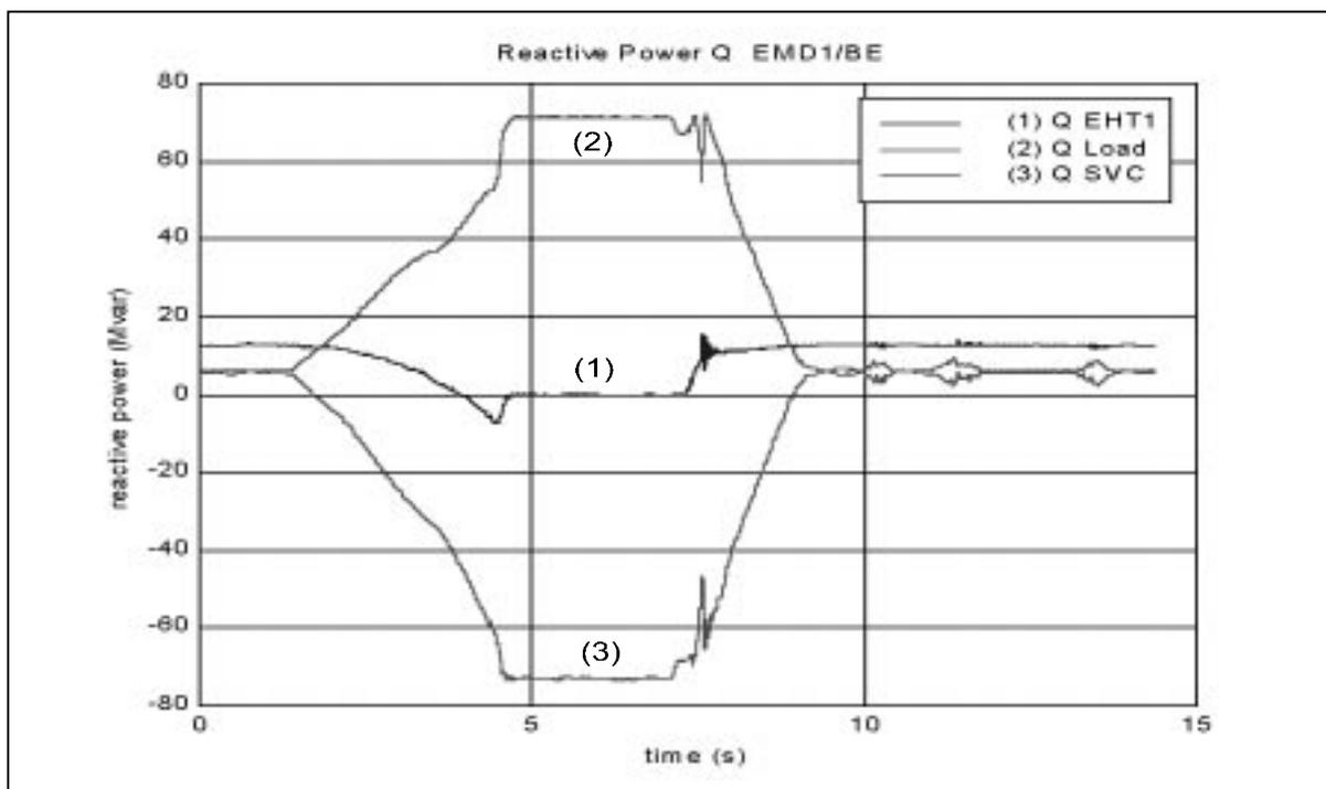
**Fig. 4:** Reactive power of pulsing load and SVC at 450 GeV.
